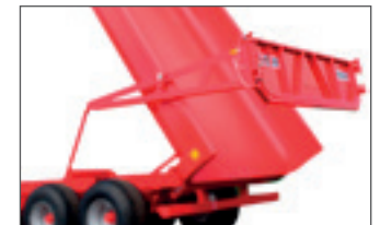
Mechanical lifting tailgate (Only for BT-8)
